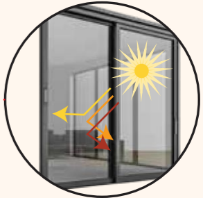
Solar Control Glass: Blocks heat letting natural light in
